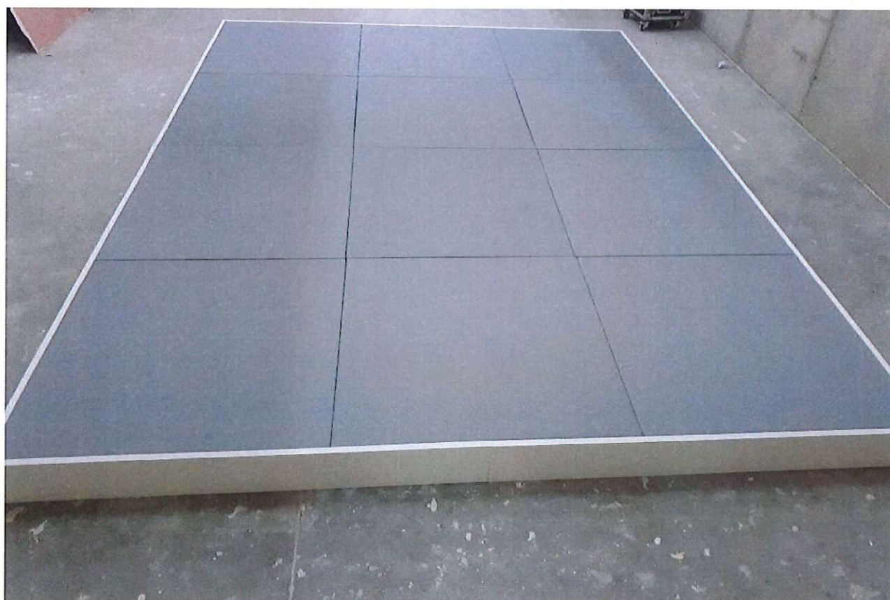
Figure. 4. Photos are presented the way of mounting of test specimen in the reverberation room. (12 panels were used). Photo Gryfitlab LA
