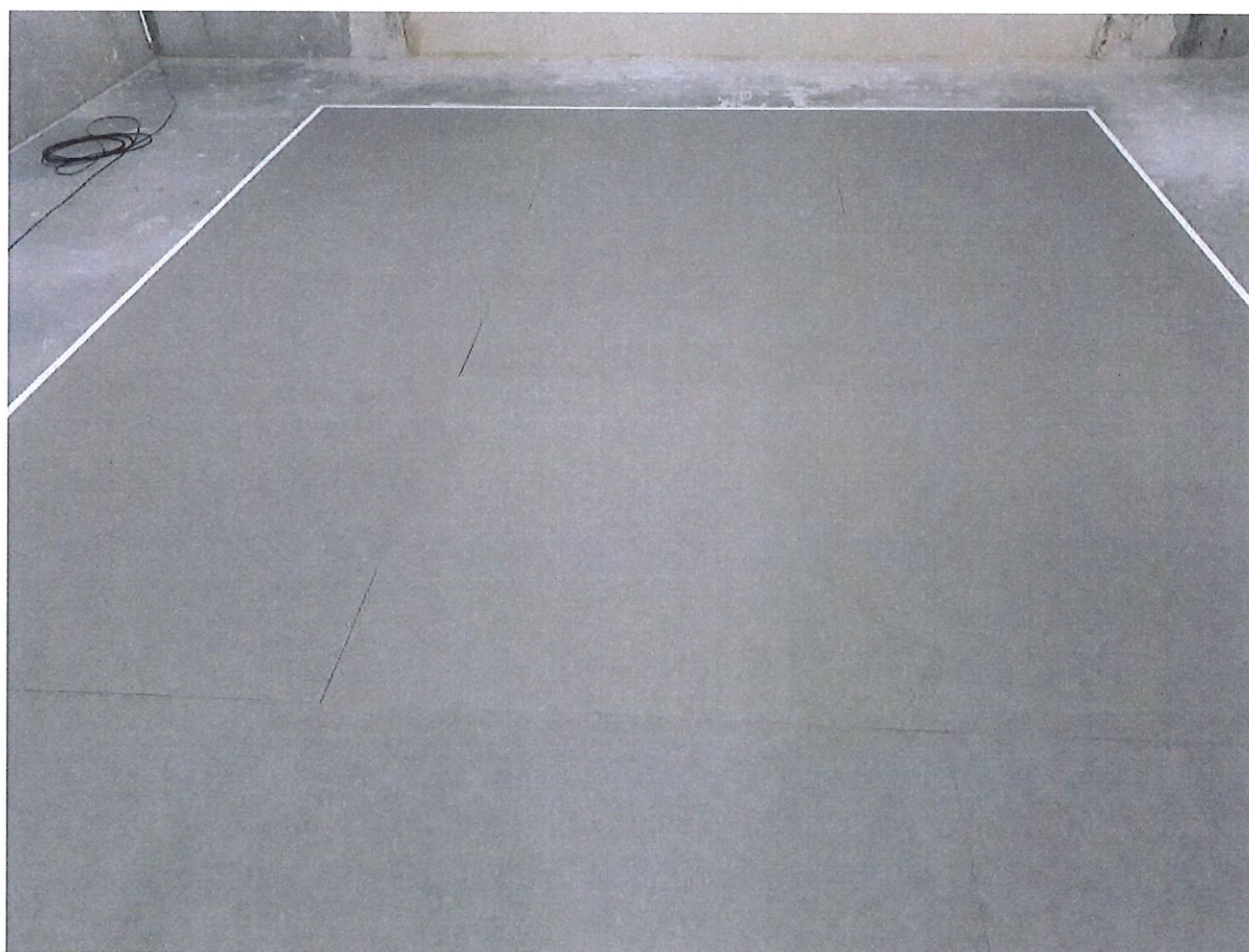
Figure. 4. Photos are presented the way of mounting of test specimen in the reverberation room. (12 panels were used). Photo Gryfitlab LA
